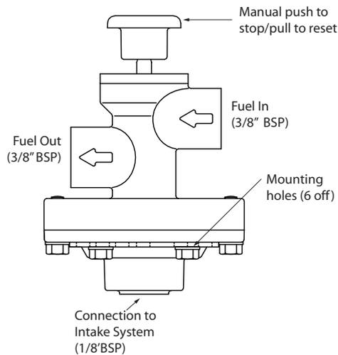
**Note.** Reset only required after an engine shut down using the air intake shut down valve or after direct manual shut down of the FSX-200.
