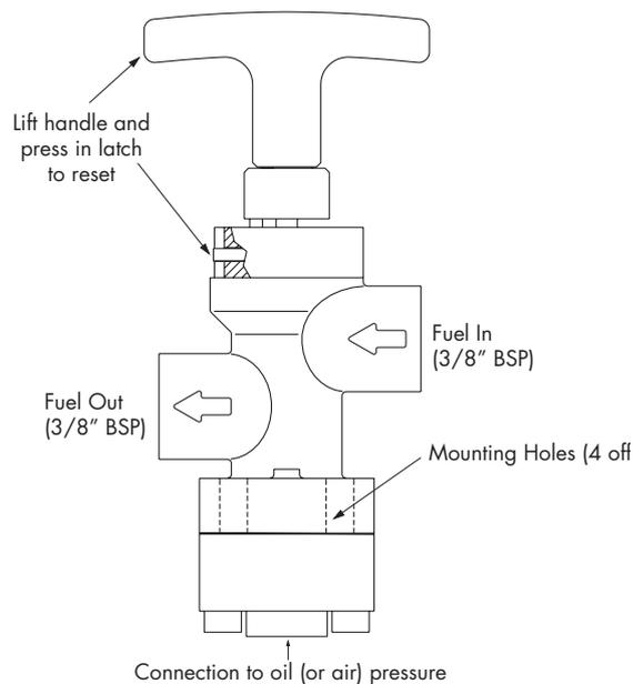
**Note.** The LST-200 normally only requires reset after an engine shut down due to the closure of the LST-200.
