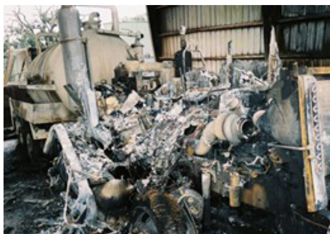
One of two trucks destroyed in a fatal accident in Texas (2003) due to engine runaway.
