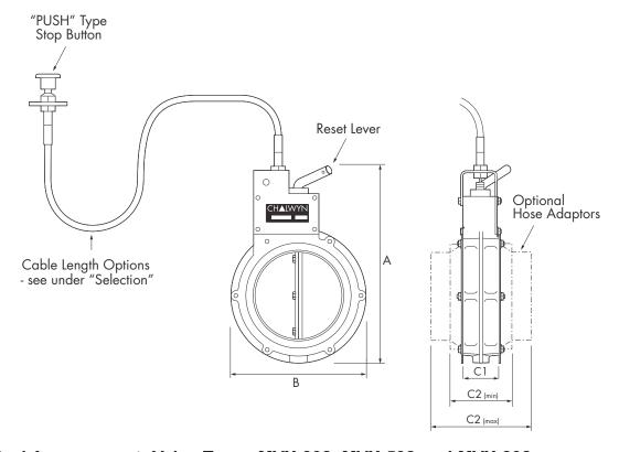
Typical Arrangement: Valve Types MVX-302, MVX-502 and MVX-802
